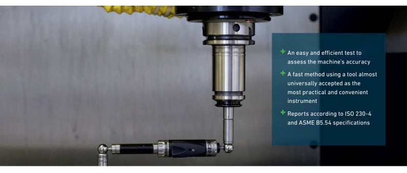
With a simple comparison of both circles, the machine accuracy is validated. If deviations are detected, recommendations will be provided for precision recovery (e.g., geometrical control, calibration by laser, components exchange).
