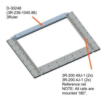
Machine table without tooling Working area:
