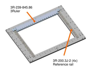
Machine table without tooling Working area:
