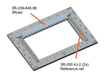
Machine table without tooling Working area:
