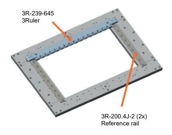
Machine table without tooling Working area:
