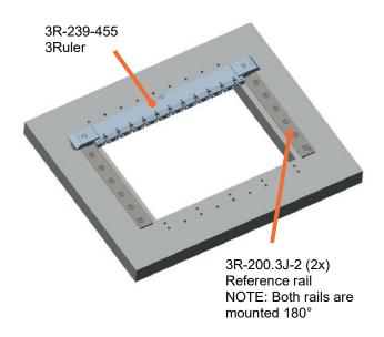
Machine table without tooling Working area:
