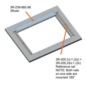
Machine table without tooling Working area:
