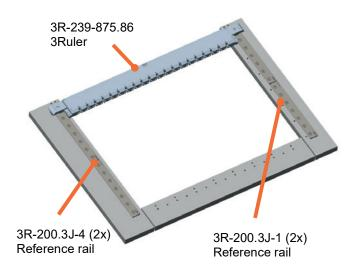
Machine table without tooling Working area:
