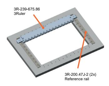
Machine table without tooling Working area:
